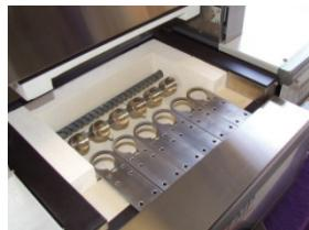
For high volume bead-making requirements, XRF Technology's six-place, electric fusion machine offers solid reliability with ease of installation and operation. These machines are capable of producing up to 30 fused beads per hour, per machine, with all functions accurately controlled and timed. Many laboratories have found that one operator can easily run two of these units simultaneously. The crucibles and moulds suitable for these machines are manufactured by our platinum labware division.
